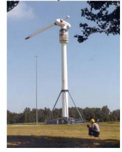
To the right you can see how NASA tested a one-bladed rotor configuration. (Photo by NASA Glenn Research Center)
